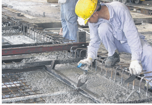
3 Concrete is poured into the mould and manually smoothed out. The component is left to dry before being removed from the mould and stored.
