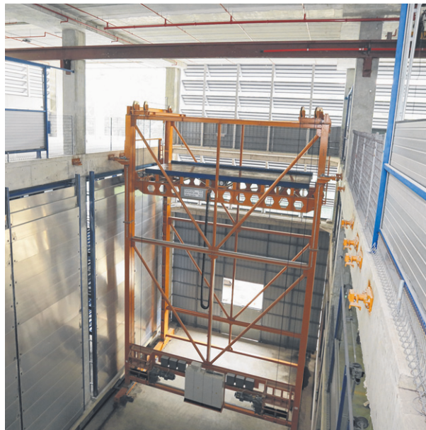
4 The concrete panel is put into a curing chamber to harden.
