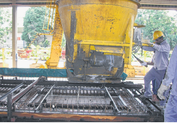
3 Concrete is poured into the mould and manually smoothed out. The component is left to dry before being removed from the mould and stored.
