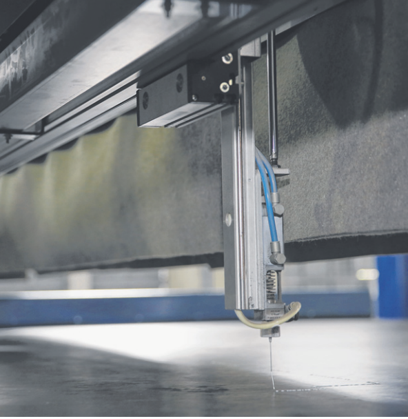
1 Using digital data from the design plans, a machine plots the required shape onto a pallet. The mould is placed on the pallet according to the plotted lines.
