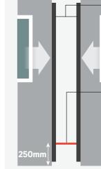
Pair of full-height mechanical safety edges
