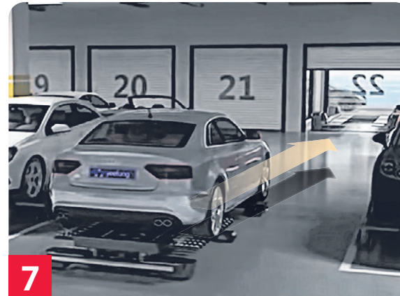
4 Guided by onboard lasers and cameras, as well as markings on the ground, the AGV can avoid obstacles, including other cars.
