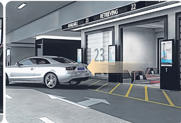
5 Able to carry cars up to a weight of 2,600kg, the platform will carry the car to an available parking space.
