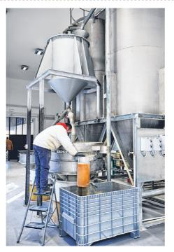
In the factory, the clay is put into a turbo mixer and sifted to remove impurities.
