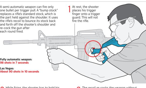
While firing, the shooter has to hold his trigger finger in place while simultaneously pushing the barrel forward and pulling the pistol grip backwards as it "bumps".
