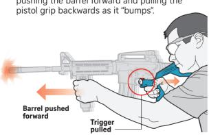
The recoil re-cocks the weapon without disengaging the trigger. Basically, the shooter can empty an entire clip by pulling the trigger just once.
