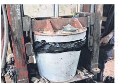
A hydraulic press is used to stamp out potshaped filters from the mixture. The pots are dried for two weeks and then fired in a kiln. This burns off fine sawdust particles, thus creating the microscopic holes for filtration
