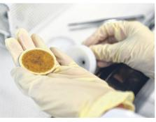
**4.** The filter pads are collected. The dark brown stains are what goes into a smoker's lungs. These substances are extracted from the filter pads using an organic solution and analysed. Any unused cigarettes are soaked in methanol to remove the nicotine before being disposed of.
