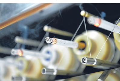
**3.** Up to 20 cigarettes are fitted into a smoking machine, which automatically lights up the cigarettes. Tar and other chemicals are collected on filter pads as the cigarettes are puffed by the machine, which has an added function of collecting and analysing the carbon monoxide produced. The lab officer has to put on a special suit to prevent inhalation of second-hand smoke.
