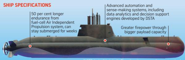
Length of Invincible 70m Surface displacement 2,000 tonnes Length of SMRT train 138m Submerged displacement 2,200 tonnes
