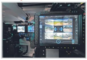
The Hunter has two three-in-one cameras – on the front and back - and three cameras on each side, to provide a 360-degree view around the vehicle. Pictured here is the display for the rear section commander, who leads the team seated at the back of the vehicle.
