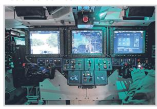
The integrated combat cockpit (pictured) seats the gunner on the left, the vehicle commander on the right, and the driver in front. An automatic target detection and tracking system allows the crew to more quickly and effectively engage targets. An upgraded command and control system, called the Artemis, allows mission planning to be done from the platoon to the battalion level.
