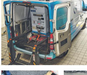
The 500 kVA generator (left) can restore electricity supply to two HDB blocks for up to eight hours.
