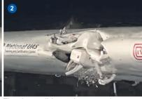
The drone did not shatter on impact but blasted a large hole in the plane's wing
