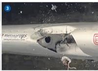
The drone lodged itself in the wing, causing extensive damage to the main structural frame or spar
