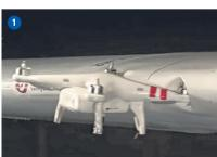
Researchers at the University of Dayton in the US fired a drone weighing about 1kg at the wing of a light aircraft at a speed of 383kmh
