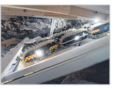
It looks like a snake and is meant to crawl through debris and rubble  Has cameras and microphones for visual and audio detection, and drops sensor units to detect chemicals such as carbon dioxide and ammonia
