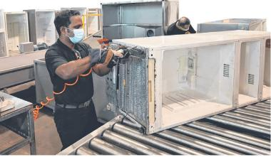
Some parts, such as the motor, will be taken to specialised machinery such as a compressor and a motor cutter, where the copper coil is extracted and then recycled.
